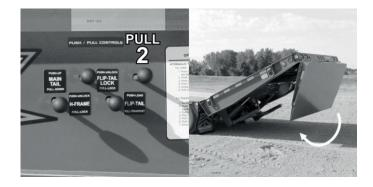
Pull the FLIP-TAIL lever to rotate the flip tail underneath the main tail section.
