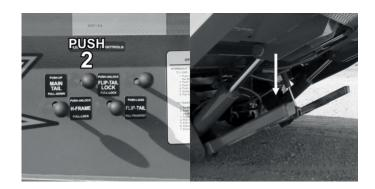
Next push the H-FRAME lever to lower the H-frame tail lock.
