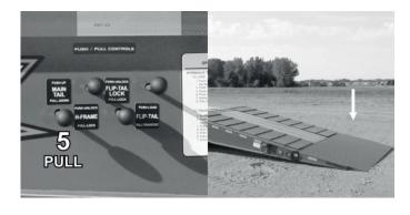
Pull the MAIN TAIL lever to lower the entire hydraulic tail for loading or unloading.
