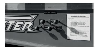
The hydraulic tail control levers are found on the neck of the trailer. The 4 levers are a push/pull type and control the hydraulic valve.
